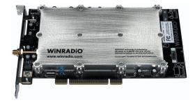
The card complies to the PCI 2.2 standard. Being only two thirds of the full PCI length, it should fit in most modern desktop computers.
